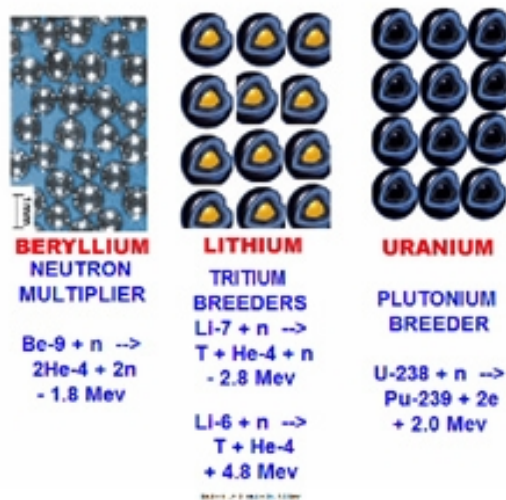
Fig III.1 Breeder blankets for fusion reactors could use TRISO packaging for layers of Lithium and depleted Uranium, using an initial layer of a neutron multiplier like Beryllium. These blankets could support a fusion reactor and 5-10 fission reactors.
