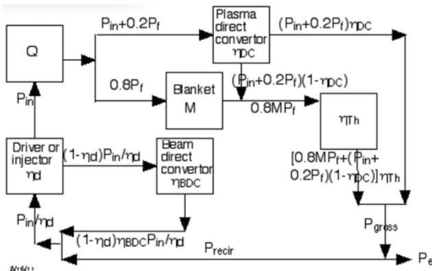
Fig. 4. Power flow diagram for axisymmetric mirror hybrid.
