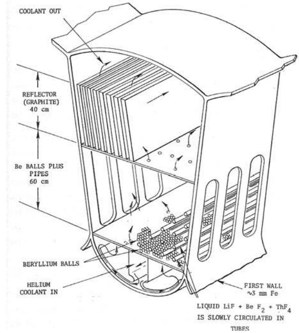
Fig. 8. Blanket submodule designed both for a tandem mirror [26] and a tokamak [27] with pebbles and helium cooling.
