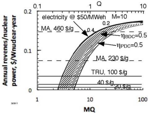
Fig. 7. Annual revenues for both actinide burning and electricity sales versus  $Q$  and  $QM$  for the actinide burning hybrid  $M=10$ .
