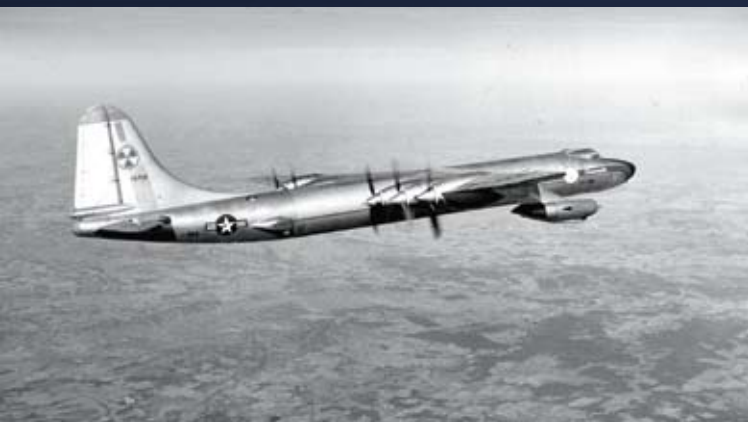
▼ The NB-36 made a number of flights in the 1950s carrying an operating nuclear reactor. The crew worked from a lead-shielded cockpit.
